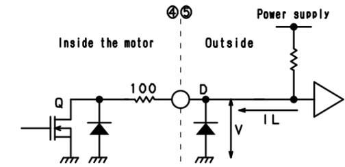
Note: Insert D (Schottky) to avoid breaking the IC by using distribution impedance.
