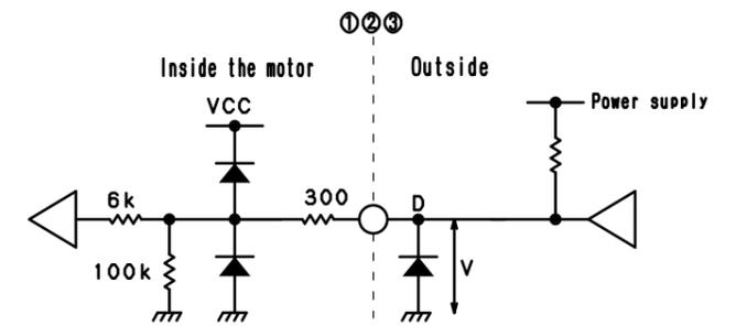
Note: Insert D (Schottky) to avoid breaking the IC by using distribution impedance.
