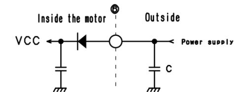
Note: The insertion C (approximately 47μF) is recommended to prevent glitches with the motor.
